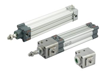
In this regard, Metal Work offers both ISO 15552 cylinders with end-of-stroke stop, which allow the rod to be retained at both ends of the movement, and the rod locks of the Secure Lock and RL Series, which allow locking even in intermediate positions.
